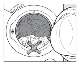
Close the drum door. To prevent damage make sure that there are no clothes caught between the drum door and seal.
